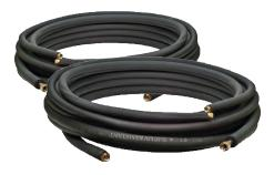
A line set is a pair of copper tubes connecting your outdoor unit to your indoor unit. The line set allows refrigerant to flow between the two units and deliver or remove heat as needed. You will typically need one line set per indoor unit, but additional line sets will be required for systems requiring a branch box.
